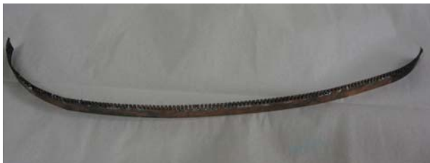
Fingerstock shouldn't look like this. When we opened the vacuum tank and smelled burned flux we knew we had a problem.
