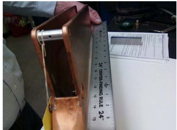
The new lower dee was installed and aligned, then removed to replace the burned fingerstock. At some point, it became bent ~2mm at the dee tip. Made of 7mm copper, it did not bend back easily. The cause is unknown.
