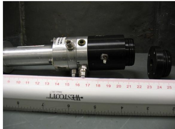
A solid target plate was prepared which had a hole drilled in the top to allow a temperature probe to be inserted to the middle of the plate. This enabled the temperature of the target plate to be monitored between the beam spot and the water cooling on the back of the plate.
