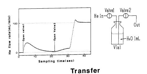
Figure 2 Typical flow rate correlation curve in transfer of 1 ml water.
