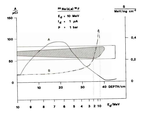
Figure 1: As the regions of maximum yield and maximum electronic heating (maximum stopping power) are separated in space, there is an optimum length of containment where the density reduction is minimized without significantly affecting the yield.
